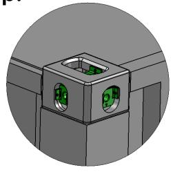
Step 2: Put corner base weldment over corner fitting. Install three 3/4"-10 bolts and thick washers. Start each by hand and then tighten with 1-1/8" socket.
