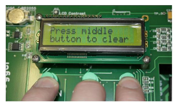
When this screen appears, release all three buttons and press the middle button. The following screen will be displayed, confirming that the internal memory is being cleared:
