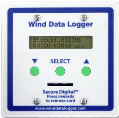
The Wind Data Logger records directly to a Secure Digital (SD™) card to provide convenient data downloads. The included SD™ card will store many years of data. The default logging interval for recording data to the memory card is 60 seconds, which is suitable for most applications; however the logging interval can range from 10 to 60,000 seconds. For your convenience, a new file is created and saved to the card for each day the logger is in use.
